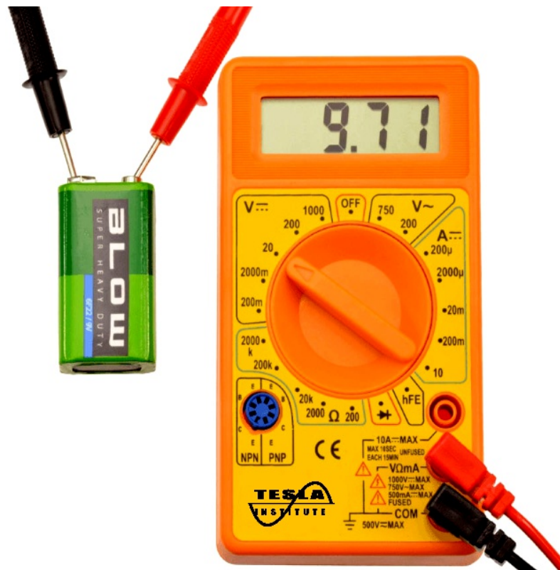
Voltage measurement on a 9V battery using a universal meter
